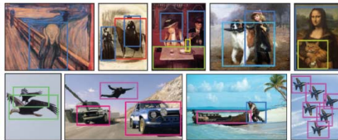
Figure 6: Qualitative Results. YOLO running on artwork and natural images. It is mostly accurate although it does think one person in an image is an airplane.
